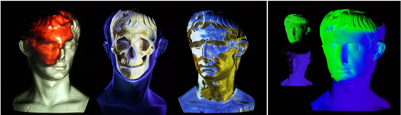
**Figure 1:** Photos of augmenting our Augustus statue (see Figure 2) with multiple projectors. First, an animated texture is projected onto the object. Second, the statue appears to be made of glass with a skull behind the surface and third, the object appears as a perfect mirror using an environment map. On the right, the contribution of the two projectors is visualized. Projector 1 is green, projector 2 is blue (see Figure 2).
