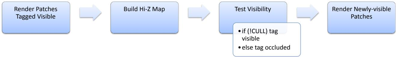
**Fig. 2** Overview of our culling pipeline within a frame: first, patches tagged visible are rendered; the resulting depth buffer is used to construct the Hi-Z map. Next, all patches are tested for visibility against the Hi-Z map. Last, all patches that were previously tagged occluded but are now visible (i.e., newly-visible) are rendered.
