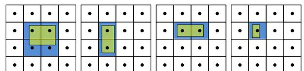
**Fig. 4** Different Hi-Z access patterns; at most four texels (blue) are chosen to cover the screen space bounding rectangle (yellow) of a patch. The case that only one texel is used (right) is special since it only applies at the finest Hi-Z level where no further refinement is possible.
