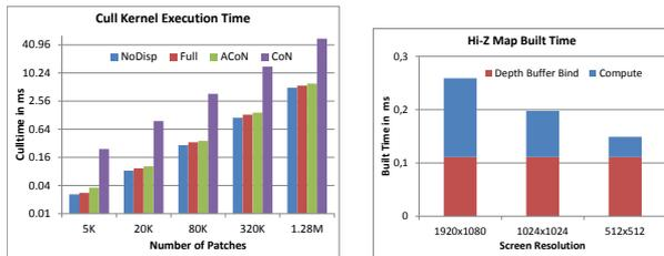
**Fig. 7** Left: execution times for different culling kernels with varying patch count. Having no displacements (NoDisp), uniform bounding volume extension (Full), and considering approximate cone of normals (ACoN) takes about the same amount of time, while using the true cone (CoN) is significantly more expensive. Right: Hi-Z map construction times for different screen resolutions. Timings are split by binding the depth buffer (depth stencil view) and running the Hi-Z build kernel.
