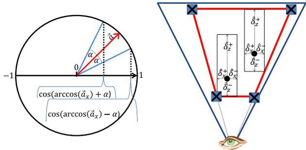
**Fig. 5** The construction of our camera-aligned frustum (CAF). Left; the cone axis  $\mathbf{a}$  and the aperture  $\alpha$  determine the extension in the positive x direction ( $\delta_x^+$ ). Right; the CAF (red) is determined in camera space for two control points.
