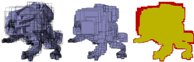
**Fig. 6** Different bounding methods for displaced surfaces visualizing object (purple) and screen space (black quads) bounds: OOB (object-oriented bounding box [10]), CAF (ours) and a comparison between OOB (red) and CAF (yellow); both using the approximate cone of normals. Our bounds generalize axis-aligned screen space bounds and thus provide optimal results for a given cone of normals.
