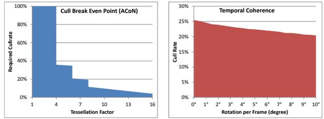
**Fig. 9** Left: required cull rates to make culling beneficial for different tess factors using the ACoN kernel. Culling becomes a win above a tess factor of 4 at a cull rate of 35.8%. Right: average cull rates using the Bigguy model for different speeds of rotation around the z-axis. Even for a large temporal change, our algorithm’s cull rate is only slightly affected.
