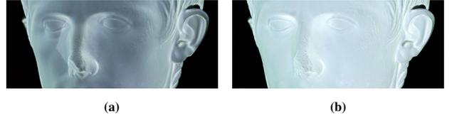
**Figure 9:** (a) Shows a multi-projection ignoring gamma correction. The sum of projected light appears too dark. (b) This effect disappears if correct gamma correction is included.
