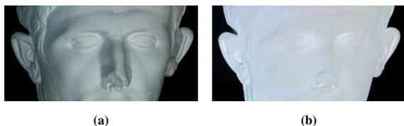
**Figure 4:** (a) Our statue illuminated with plain white light from two projectors. (b) The statue illuminated from both projectors when compensating for Lambertian attenuation, distance and overlap.
