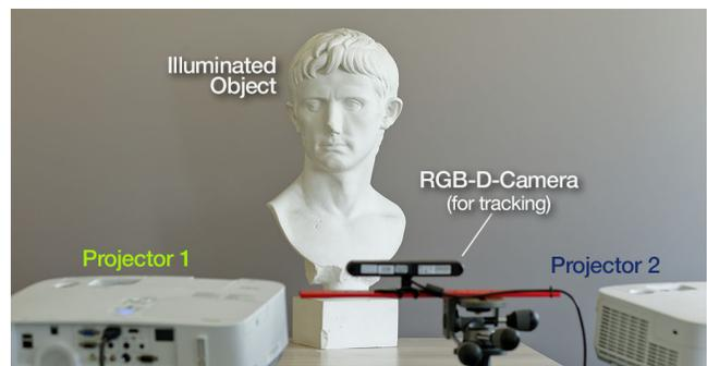
**Figure 2:** Our primary setup: Projector 1 projects from the chin upwards, projector 2 from the temple downwards. In the overlapping regions both projectors can illuminate the statue.
